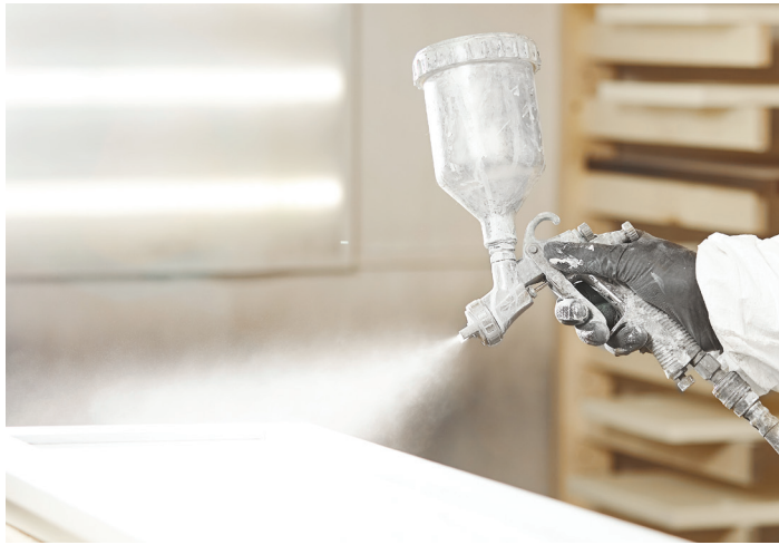
Use an HVLP spray gun with a fine-finish tip for spray applications.
