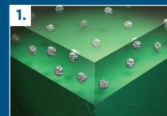
The substrate is top coated with Eco Spec<sup>®</sup> WB Silver, which contains EPA-approved antimicrobial agents including elemental silver. The silver molecules are imbedded within the paint.
